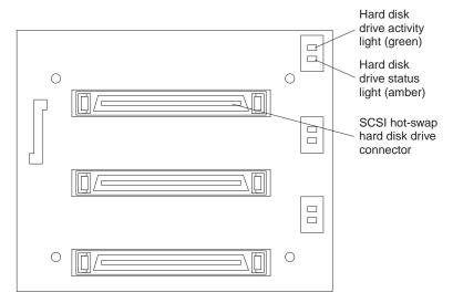
**Note:** The hard-disk drive activity light and hard-disk drive status light on the backplane match the hard-disk drive activity light and hard-disk drive status light on the front of the server (see "Start the server" on page 8).
